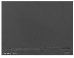
Fig. 3 – SEM analysis: the Er:YAG laser irradiation achived a complete removal of contaminats on implant surfaces
